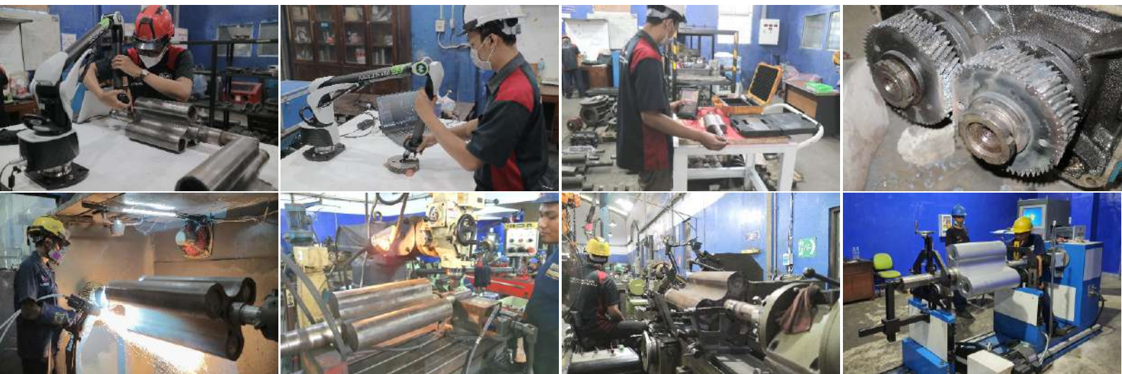
Roots Blower Rotor Gear, Analysis , Repair & Balancing Process
