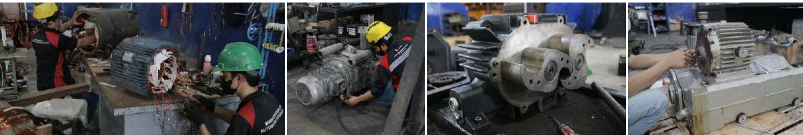
Motor Rewinding Process
