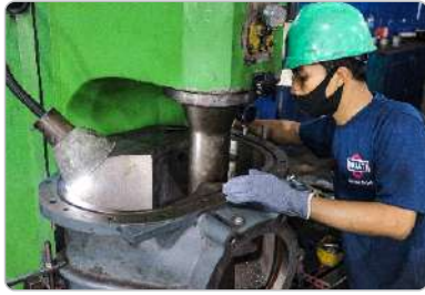
Vertical Line Boring
